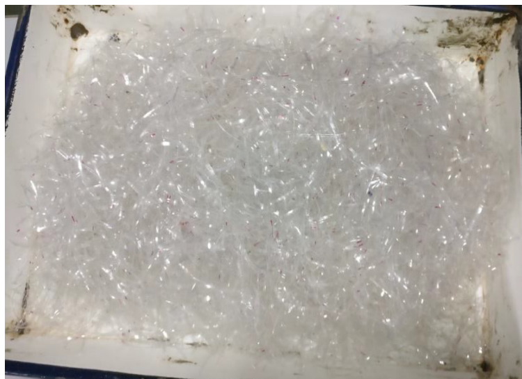
Fig. 1 Fibers of aspect ratio 50mm x 2mm
