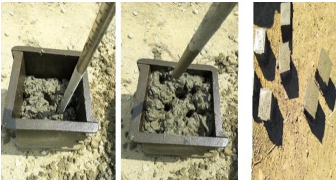
Figure 2: Cube casting (step by step) for trail mix
