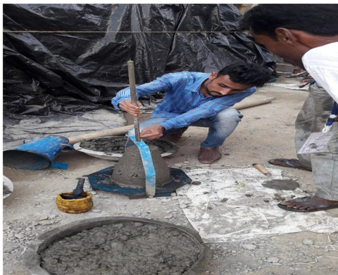
Figure 1: Slump Testing for workability
