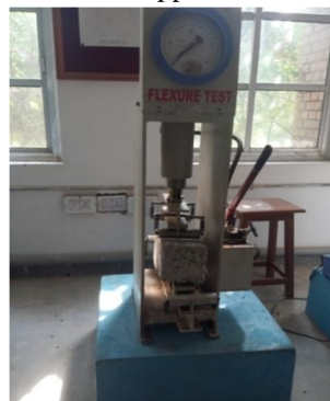
Figure 4 Flexural Strength Test Apparatus
