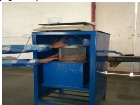
Figure 2 Wire bucket for Specific gravity
