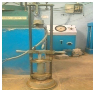
Figure 1 Aggregate Impact Test Machine
