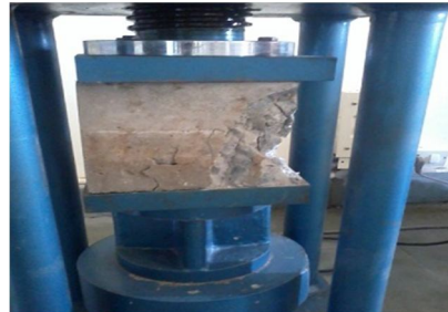
Figure 3 Crushing strength test
