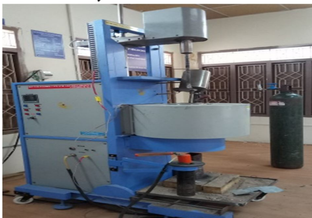
Fig.5. Bottom type Stir casting equipment
