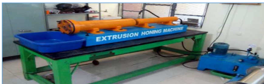
Fig 1: one way type of extrusion honing Machine
