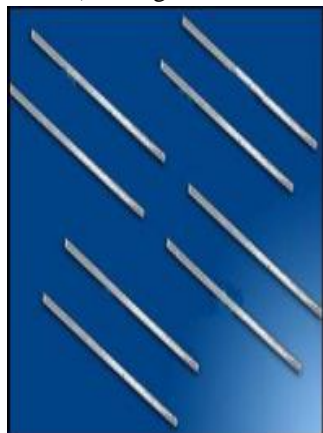
a) Straight Slit Steel fiber
