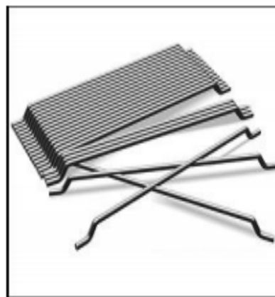
b) Hooked End Steel fiber
