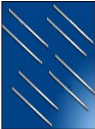
a) Straight Slit Steel fiber
