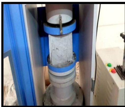
Figure 6: Cube under compressive test
