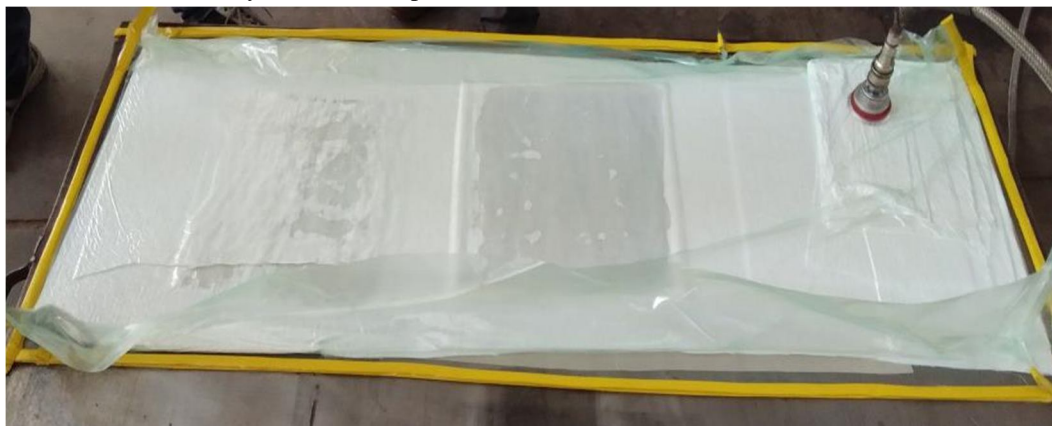
Fig.14 Vacuum Bagging of Laminate
