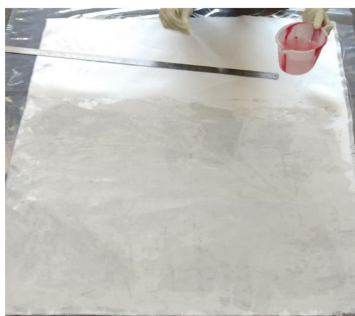
Fig.12. E-glass Fabric with Epoxy Resin Hand Layup
