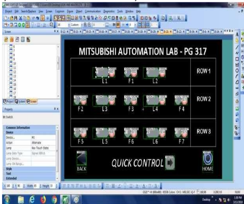
Fig.5.HMI screen for individual control
