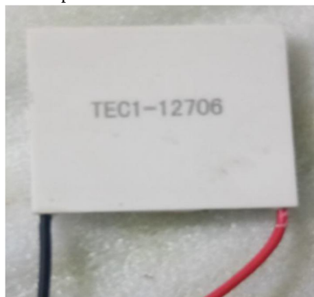
Fig. 3.1. Sample of peltier module (procured)
