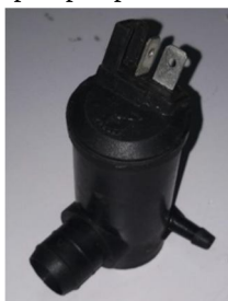
Fig. 3.6. Pump for coolant recirculation (procured)
