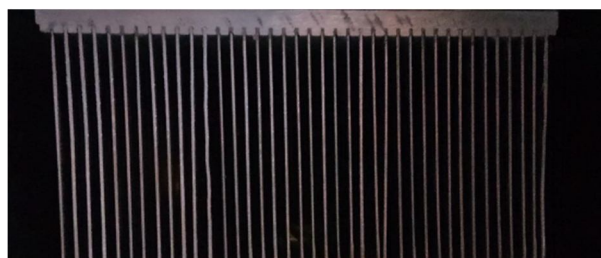
Fig.3.3. Cooling fin for inlet air cooling
