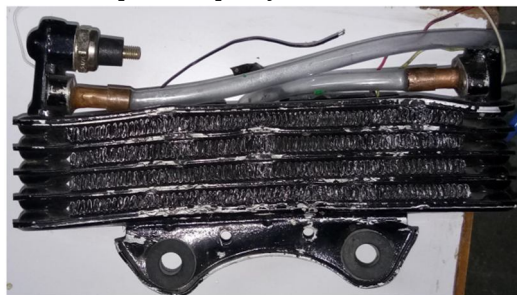
Fig. 3.4. Radiator to drop temperature of coolant (procured)
