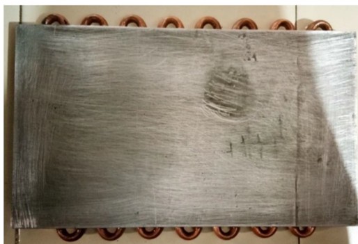
Fig. 3.2. Perforated block heat exchanger (fabricated)
