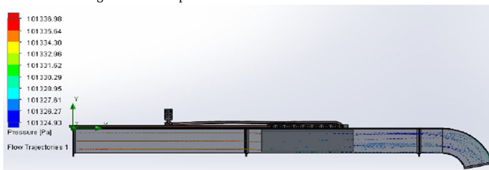
Fig. 2.16. Pressure loss in inlet duct
