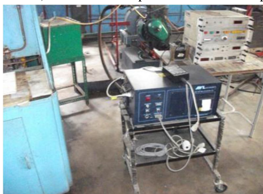
Fig. 2.4 AVL smoke and emission analyzer
