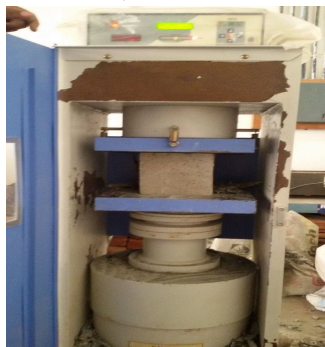
Fig. 2 Testing cubes for its compressive strength.
