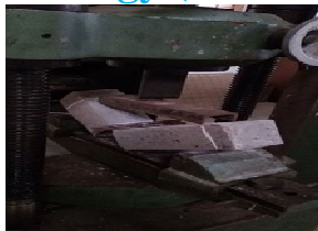
Fig. 4 Testing of beams for its flexural strength.
