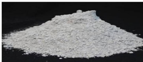
Figure 3.1: Lime Stone Powder
