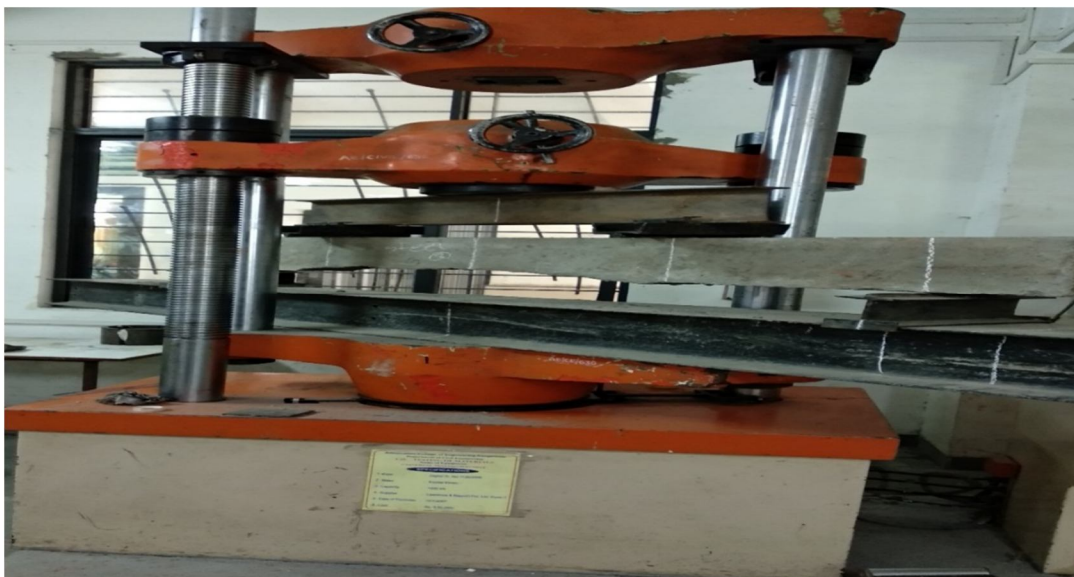
Photo 3 Two point loading set up
