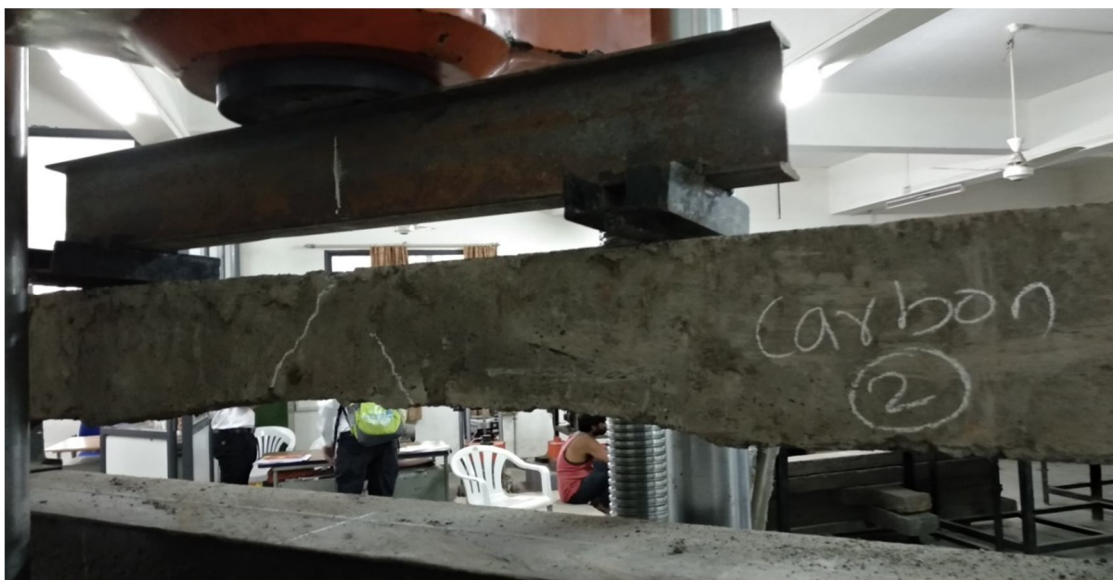
Photo 2 Testing of Haunched Beam
