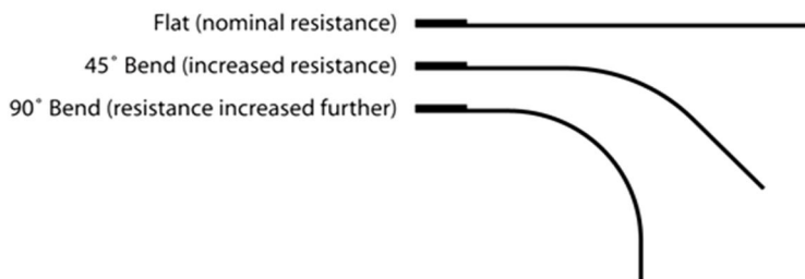
Fig.4 Flex Sensor Resistance Diagram
