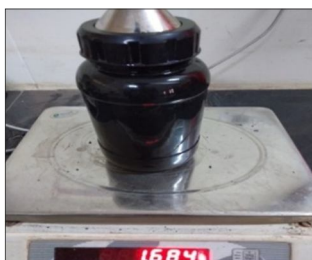
Fig. 3.2.1: Pycnometer filled with carbon black powder & water
