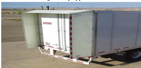
Base plates and side plates attached to the trailer rear end.
