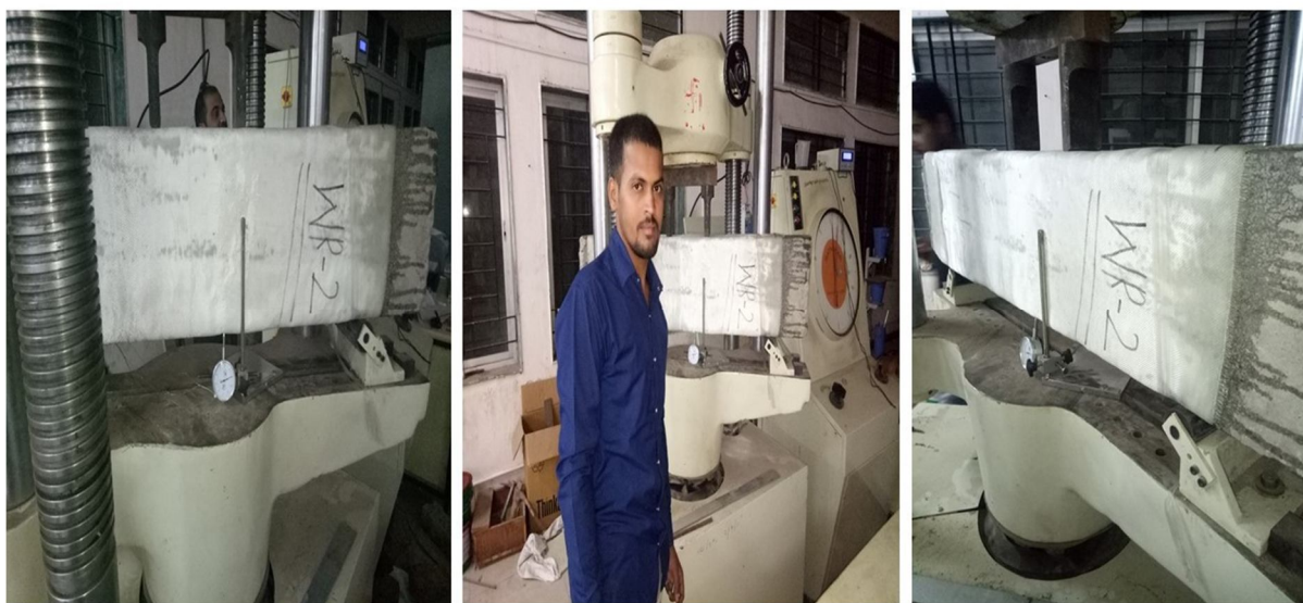
Fig.6. Testing of GFRP retrofitted RC beams
