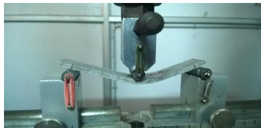
Figure.1 Flexural testing of the specimen (ASTM D 790). Figure 2. Load vs. displacement graphs for flexural test (ASTM D 790)
