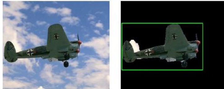
Figure 9 . Effect of Grab-Cut algorithm
