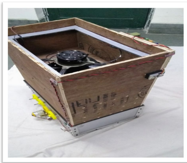
Figure-3 Final assembly of Purifier
