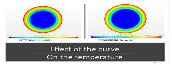
C. Variation of Temperature along Heat Exchanger
