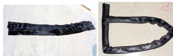
Fig 3.4 A tube like structure is made from two piece of synthetic rubber sheet and it is inserted through the multi-wood strip.
