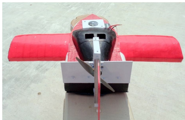
Fig 3.10 Rudder is fixed on the rudder mount.
