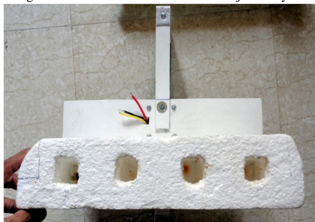
Fig 3.9 The multi-wood with thrust motor is fixed on a rectangular form, and tightened with screws
