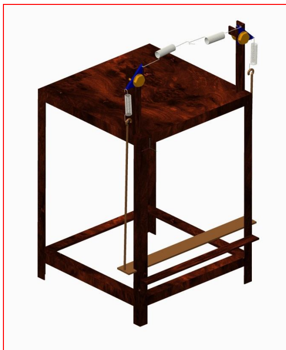
Fig.3 CAD Model of Foot operated Round Ring Cloth Peg Assembly Machine
