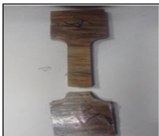
Fig 1 : Sample A 60% coir and 40% kenaf
