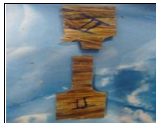
Fig 2 : Sample B 60% kenaf and 40% coir
