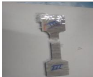
Fig 3 : Sample C 60% jute , 40% kenaf
