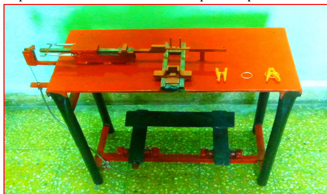
Fig.3 Foot operated Round Ring Cloth Peg Assembly Machine
