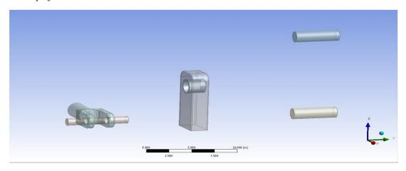
The source design of our project is to design the part between the pins and the hydraulic arm. The cylindrical shaft is drawn through the rectangular block.
