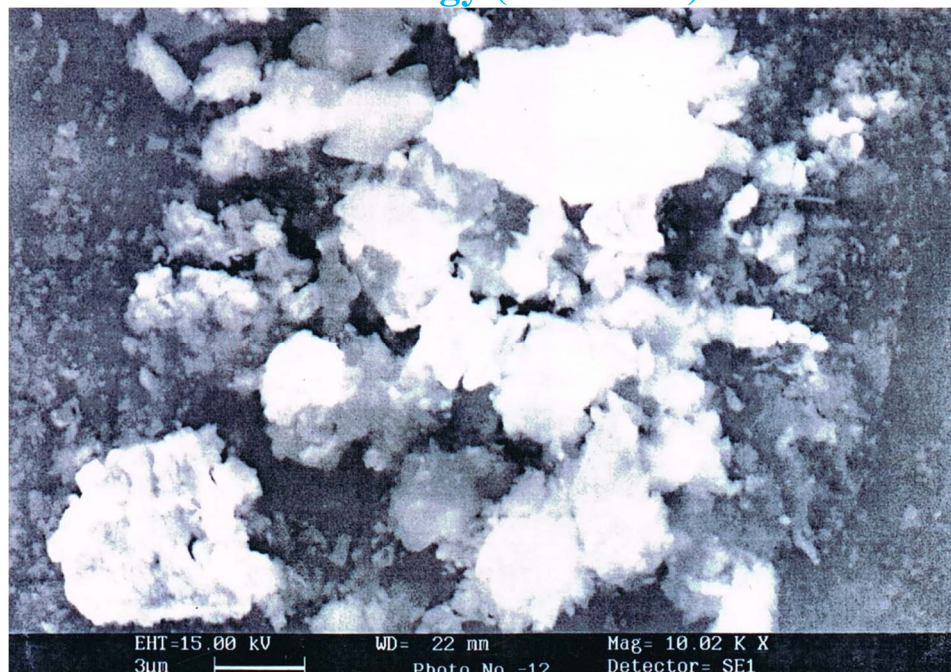
Fig.4. SEM image of Pani/CdS thin film on to glass substrate.
