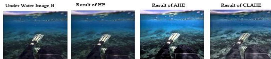
Fig: Performance of HE, AHE, CLAHE on Underwater Image B
