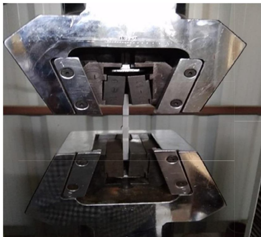
Fig. 5 Welded sample before tensile test.
