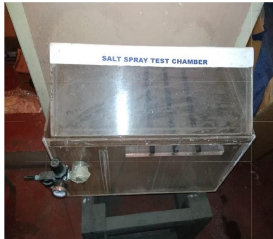
Fig. 7 Salt spray test chamber.
