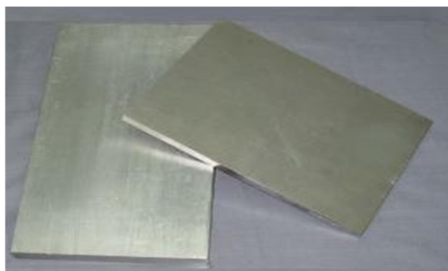
Fig 1.1 Aluminium Alloy 6063-T6
