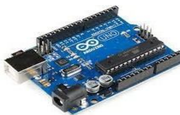
Figure 1.5 Arduino-UNO (ATMEGA328 Microcontroller) Systems.
