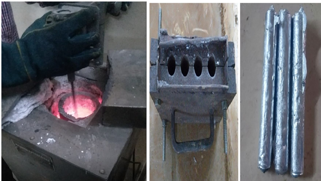
Fig 1.1 stir casting, Cast Iron Die and fabricated samples
