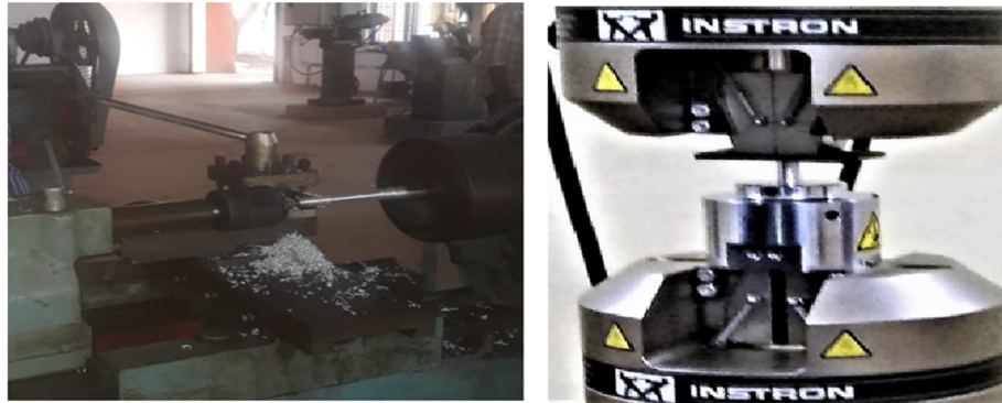
Fig 1.2 Machining the casted samples & Testing on UTM(Instron)
