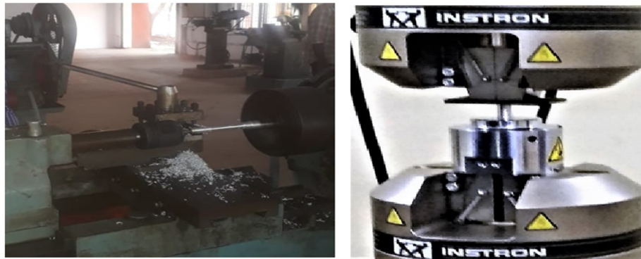
Fig 1.2 Machining the casted samples & Testing on UTM(Instron)
