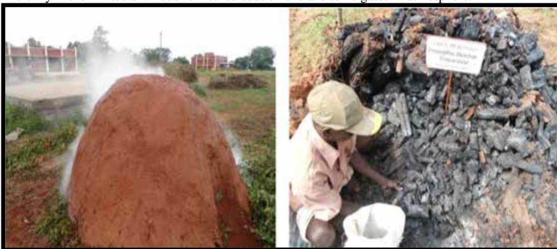
Figure 4: Heap method of biochar preparation in Tamil Nadu. (Source- NICRA Bulletin 1/2013)
