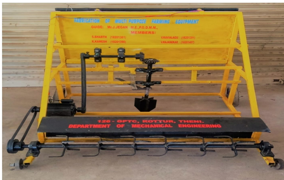
Fig 4.2 Fabrication of Multipurpose Farming Equipment
