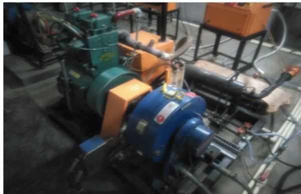
Figure1: Computerized Diesel engine test rig
