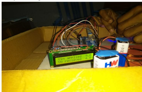
Figure 5: LCD showing the measure of voltage transferred between transmitter and collector.
