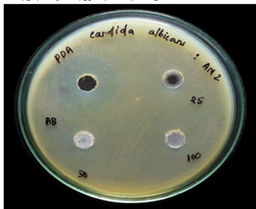
Fig.11. Activity of [Mn(dafone) 2 (CH 3 OH) 2 ] 2(ClO 4 ) 6H 2 O against the fungus Candida albicans
