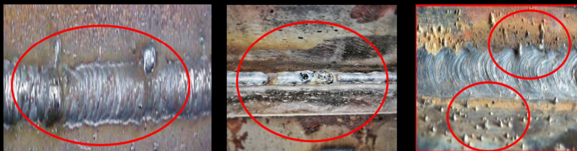
Figure 4 – Defects Observed in Rejected Welding Samples (S1) Taken (without paint)
