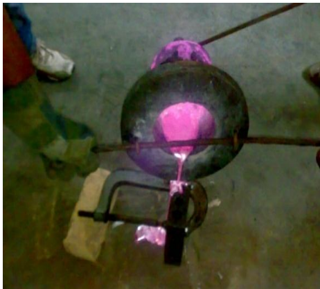
Fig. 4 Pouring of Molten metal into die
