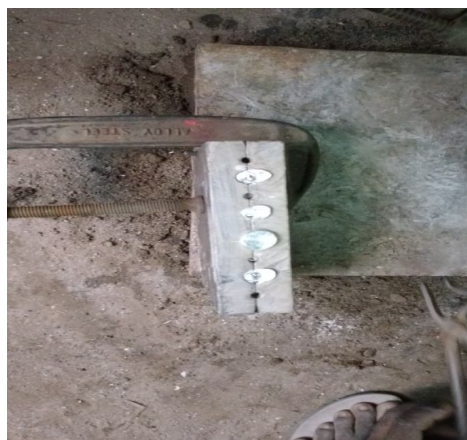
Fig. 5 Casted specimen in the die
