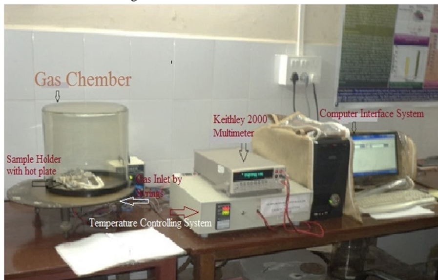
Fig. 3 Gas sensing setup used in present work
