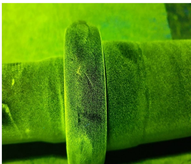
Fig II. 5 Crack detected under UV Light
