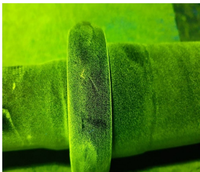
Fig II. 5 Crack detected under UV Light
