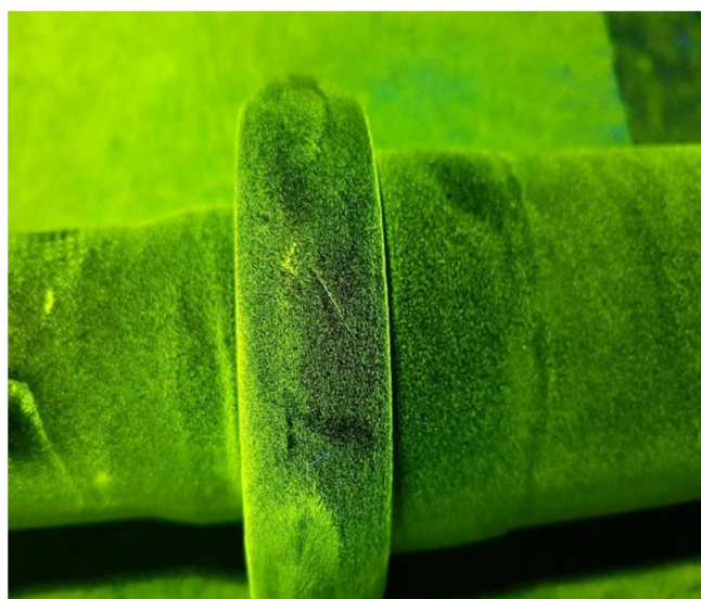
Fig II. 5 Crack detected under UV Light
