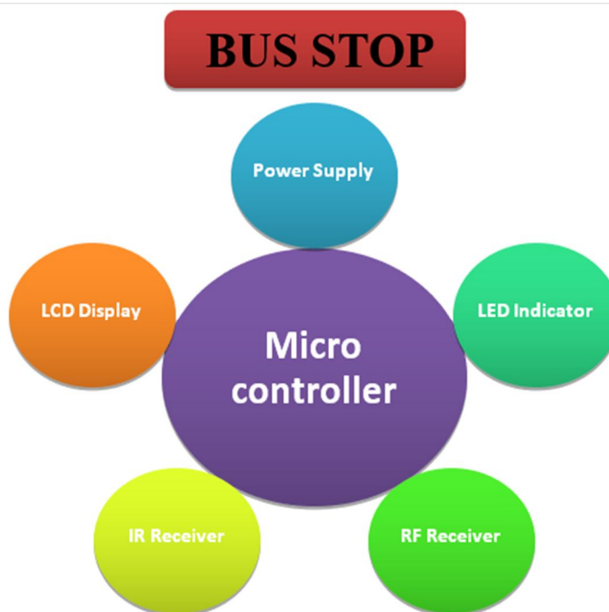
Fig. 2. Block dig. Of Bus stop section.
