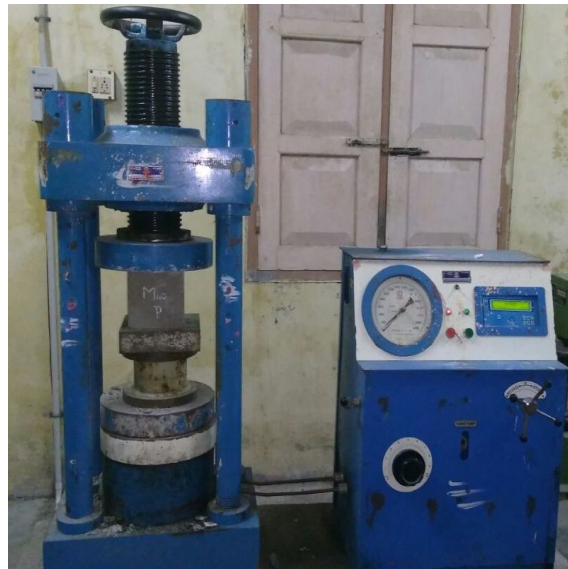
Fig.3 Compression test on concrete cubes
