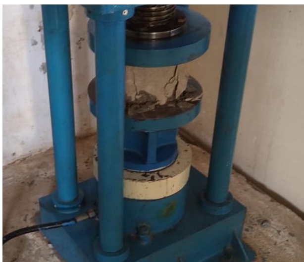
Fig.5 Failure of cube specimen
