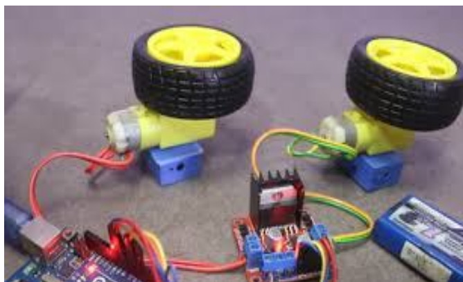
Fig.6 DC Motor Controlling using L298 Motor Driver
