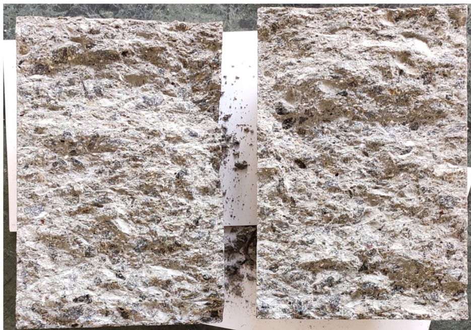
Fig.5: Failure pattern of specimen
