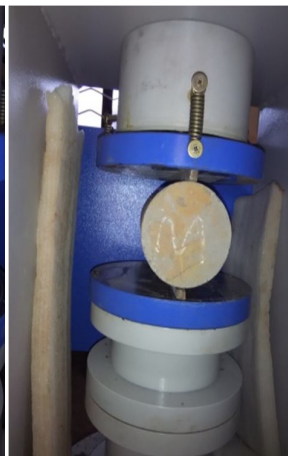
Fig 3: Split Tensile Strength Test
