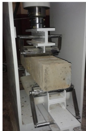
Fig 4: Flexural Strength Test
