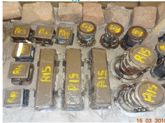
Fig 1: Moulds filled with concrete
