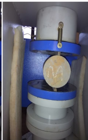
Fig 3: Split Tensile Strength Test
