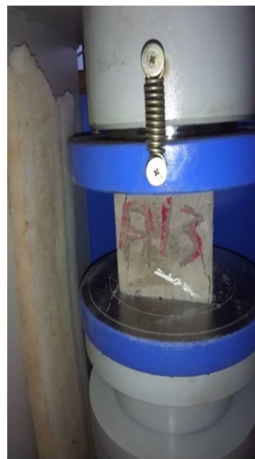
Fig 2: Compressive Strength Test
