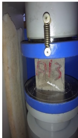
Fig 2: Compressive Strength Test
