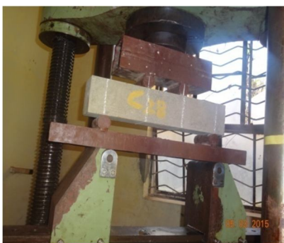
Fig 4: Setup for Flexural Strength Test
