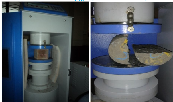
Fig 2 & 3: Setup for compressive and split tensile strength.
